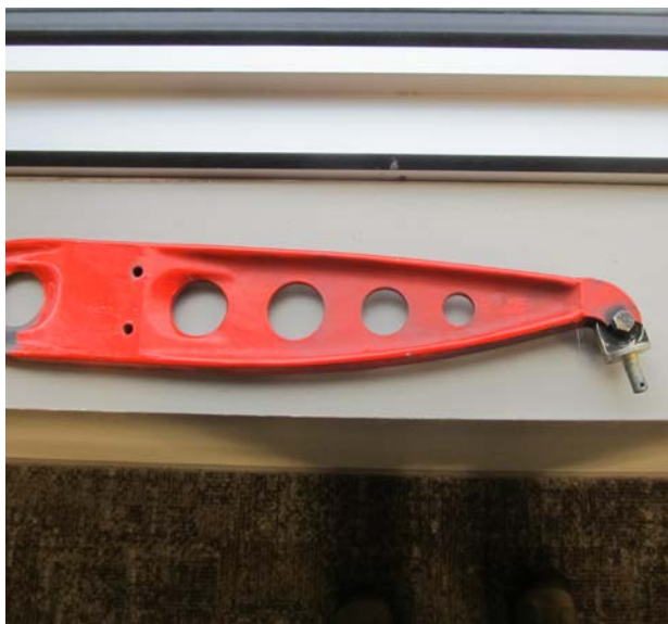
Hinge with missing piece
